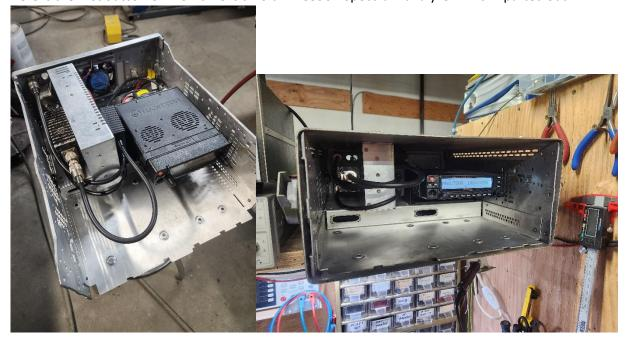
Using here a Wouxun KG-UV920P-A dual band radio, Meanwell 30A PSU and a Diamond Triplexer (all I had around).
