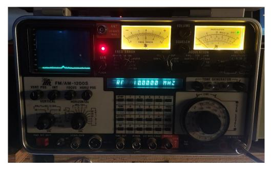
Sometimes the shop can be dark or weird light reflection coming onto the analog meters. Opened the IFR and looked around where a good place would be for additional lightning. Found a perfect hole which will hold a 3mm LED. Applied hot glue around LED and inserted it into the board. Let it try up and don't burn your fingers while holding HIHI Add resistors to LED's, add heat shrink, wires and connect it to the power supply board. LED's used are warm white.
