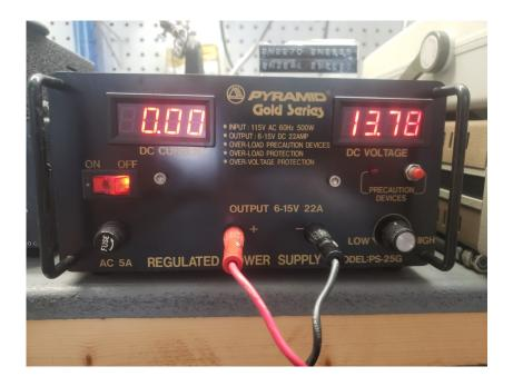
The next step was to replace the standard voltage control pot with a 10 turn one. I found the standard pot was a bit too touchy for any sort of precision.
